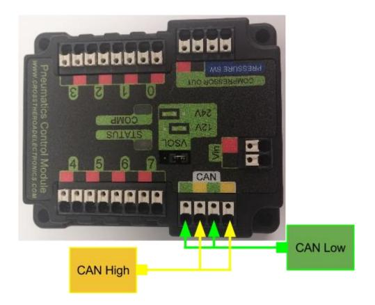
Weidmuller Connectors are also used for CAN Communication. See <u>Section 2.1. Weidmuller</u> <u>Connectors</u> for for wire insertion and removal procedures. PDP provides termination and may be placed at the end of CAN bus chain.
