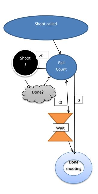
State 1: maxBalls = passed in value (e.g. 2) askRobot = passed inv value (e.g. true) save passed in timer reset timer have ball state:
